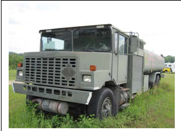
Truck Tank (Refueling) 6,000 gallon 6x4
